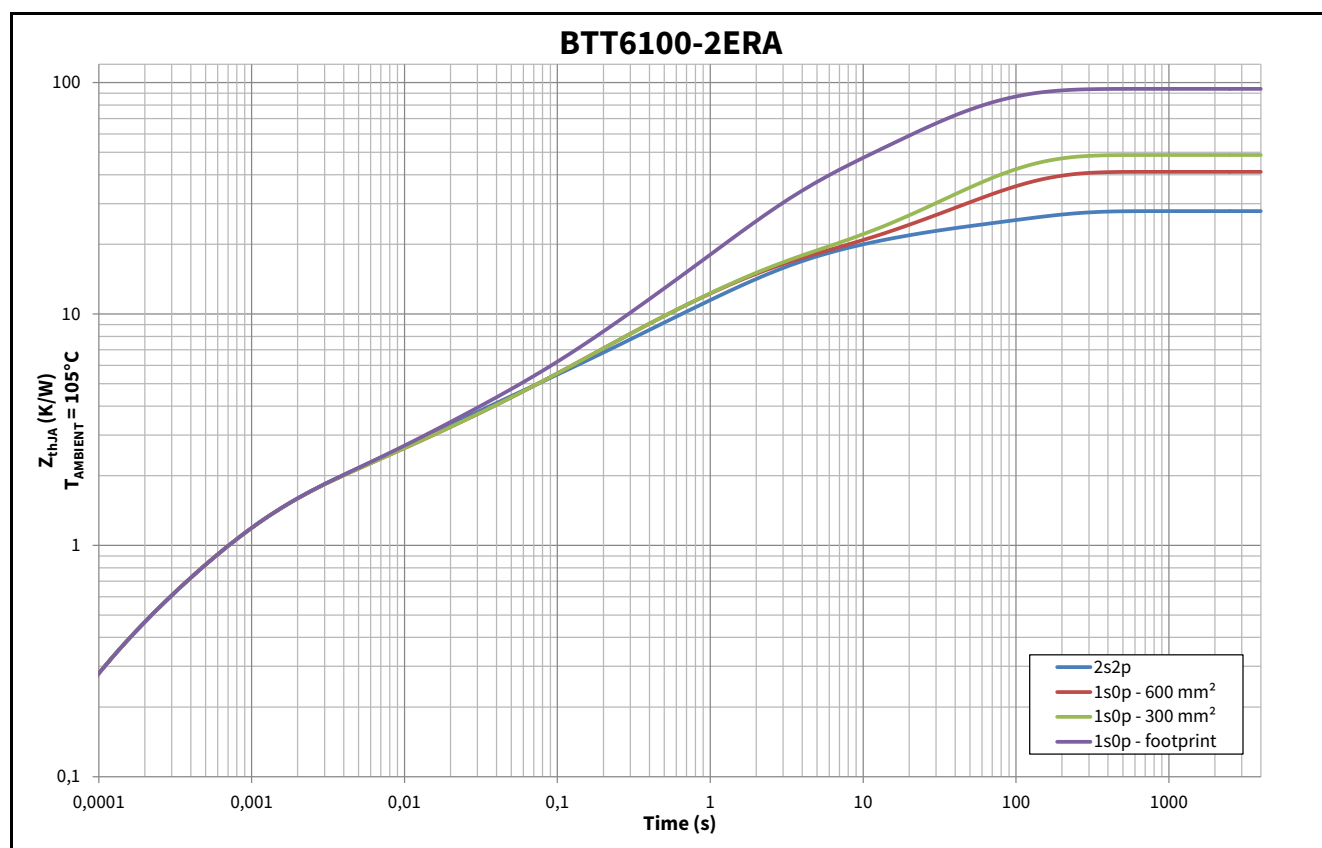
Figure 6 Typical Thermal Impedance. 2s2p PCB set-up according to Figure 5
